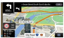
There is a field in the top left corner displaying the next manoeuvre. Both the type of the manoeuvre (turn, roundabout, exiting motorway, and so on) and its distance from the current position are displayed.
