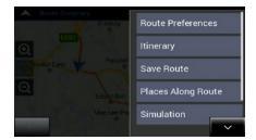
4. Tap Simulation Simulation starts from the starting point of the route and leads you through the whole planned route using a realistic speed.
