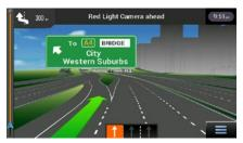
Where Provider Junction Views are not available but the necessary information exists, <u>Generic Junction Views</u> show a generic view of the junction, focusing on the number and layout of lanes only. The road signs are created from road shield, road number, and destination information received in the map data.
